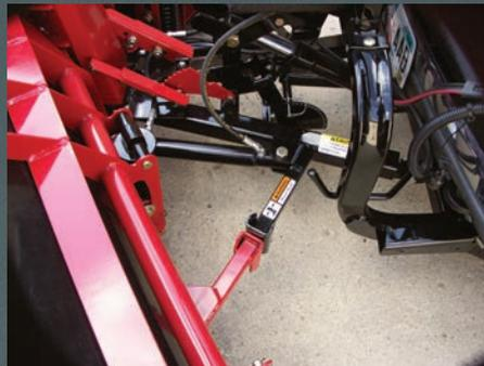
**Positive wing stops** relieve stress on the hydraulic cylinders. 2-way cylinders provide precise moldboard control.
