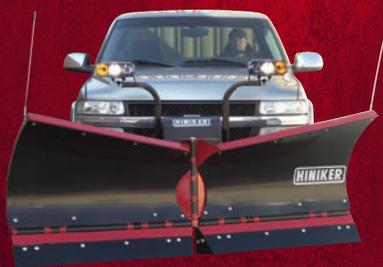
**Double-acting cylinders** provide positive hydraulic control of moldboard position, whether plowing forward or backdragging.
